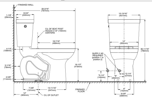
\* THIS COMBINATION IS DESIGNED TO ROUGH-IN AT A MINIMUM DIMENSION OF 305MM (12") FROM FINISHED WALL TO C/L OF OUTLET.
